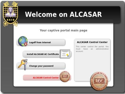
The main page allows users to log-off, to change their password and to import the security certificate into their browser. It allows administrators to manage, in secure way, the portal via the Alcasar Control Center (ACC).
