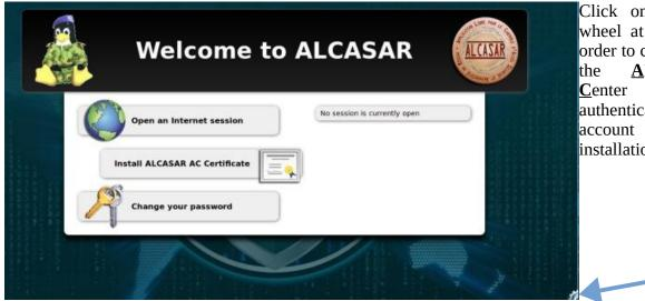
Click on the small cranted wheel at the bottom right in order to connect via HTTPS to the <u>A</u>LCASAR <u>C</u>ontrol <u>C</u>enter (ACC). You must authenticate you with the first account created during the installation process.
